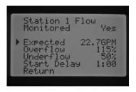
Expected Flow may be changed manually in this screen, or you may relearn any of the stations flow by repeating the process just discussed. This will be necessary if additional heads have been added, heads have been removed, or nozzles have been changed to a station, which will all adjust the flow.
