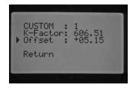
may be changed, press the +/- button to either increase or decrease the value. Once you have completed entering the K-Factor and Offset specified by the manufacturer of the flow sensor, use the  $\blacktriangledown$  button to return to the main Sensor Configuration screen.
