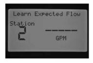
a minute. Once the controller has Learned Expected Flow the controller will shut the stations down and the controller will go back to the main current date / time screen.
