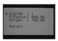
the value. Once you have completed entering the K-Factor and Offset specified by the manufacturer of the flow sensor, use the ▼ button to return to the main Sensor Configuration screen.
