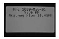
the station running, the controller will acknowledge that there is flow, and the Flow Status light will light solid RED, indicating an unscheduled flow.
